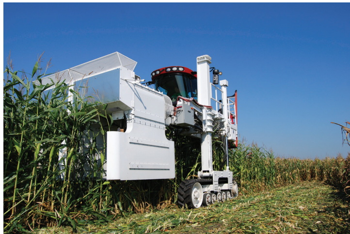
Figure 4. Corteva Agriscience's Boreas wind machine creates winds that can exceed 100 miles per hour to test for brittle snap resistance and standability in corn hybrids.
