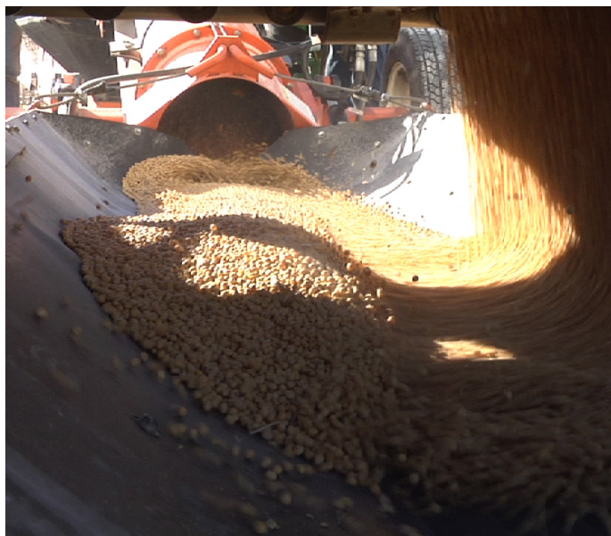
Soybeans being unloaded from the truck hopper onto a belt conveyor. Belt conveyors are designed to more gently handle seed.
