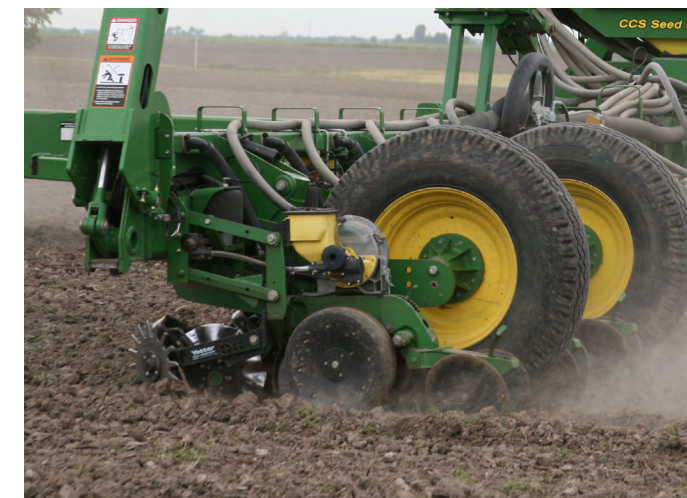
Replacing worn parts and ensuring all components of the planter row units are performing properly are critical for achieving uniform seed placement and good seed-to-soil contact.
